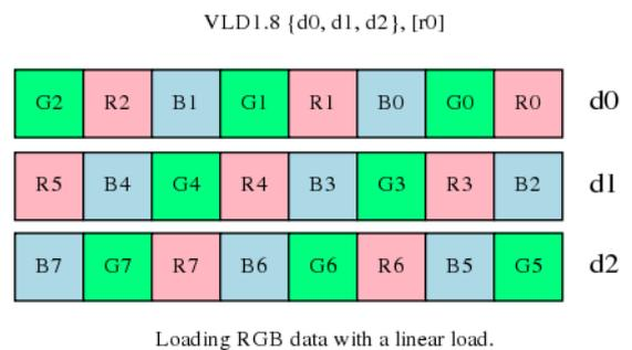
**Figure 6-1 Loading RGB data with a linear load**
