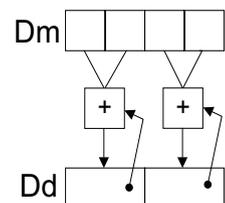
**Figure C-39 Example of operation of VPADAL (in this case for data type S16)**
