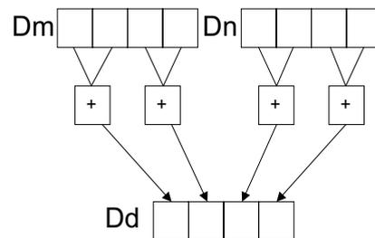
**Figure C-37 Example of operation of VPADD (in this case, for data type I16)**
