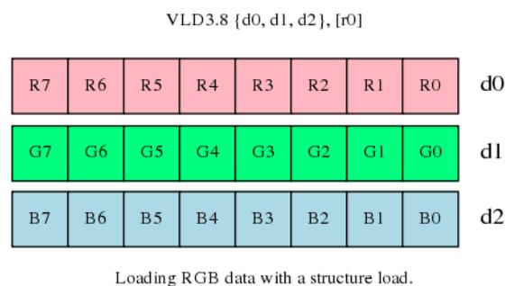
**Figure 6-2 Loading RGB data with a structure load**
