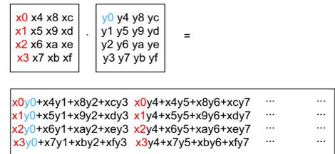
Figure 7-1 Matrix multiplication showing first two columns of result
