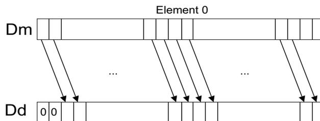
Figure C-18 Operation of doubleword VSRI.64 Dd, Dm, #2
