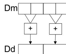
**Figure C-38 Example of operation of doubleword VPADDL (in this case, for data type S16)**
