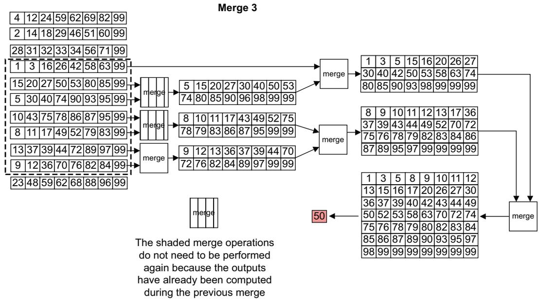
Figure 8-11 Merging 7 vectors for third median pixel
