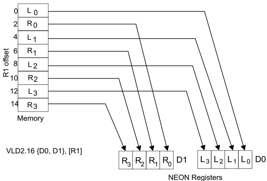
**Figure 5-1** Labeled example of load de-interleaving
