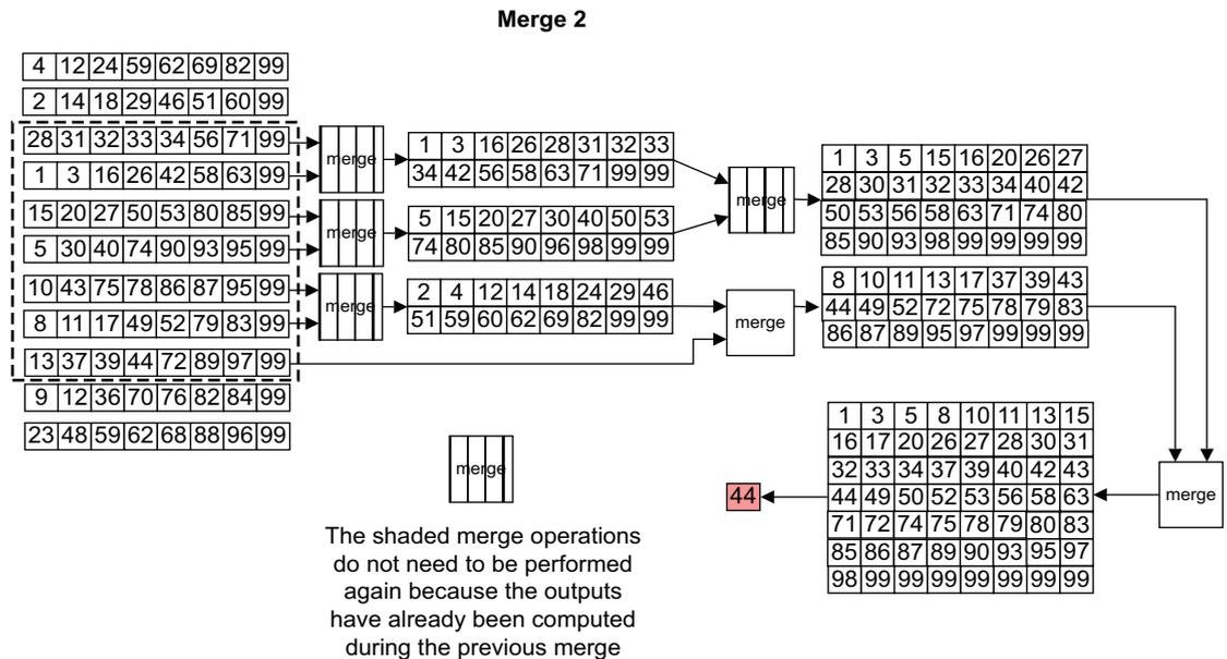
Figure 8-10 Merging 7 vectors for second median pixel
