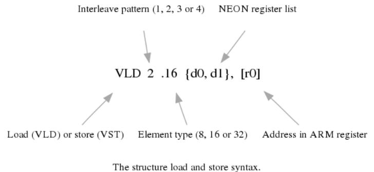
**Figure 6-5 The structure load and store syntax**
