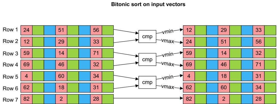
Figure 8-5 Comparing corresponding elements of input vectors
