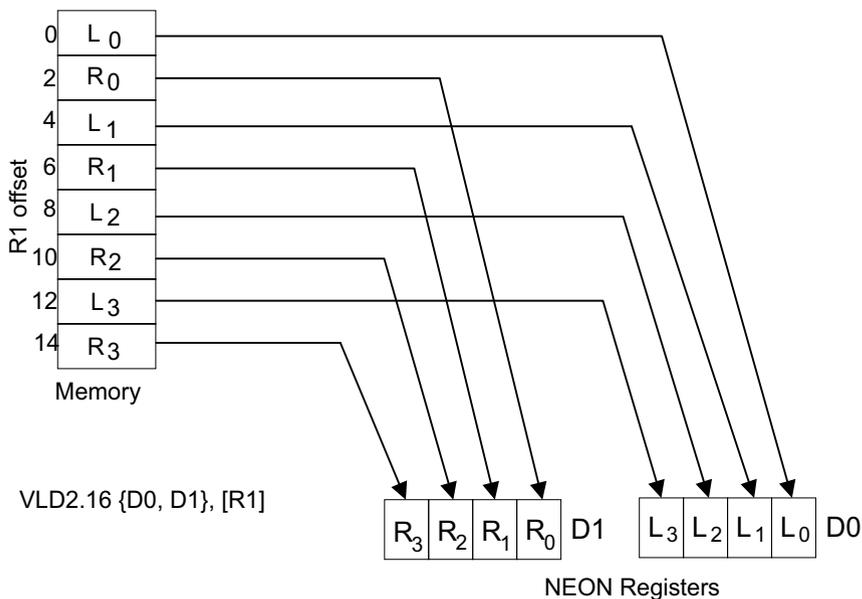
Figure C-48 De-interleaving an array of 3-element structures
