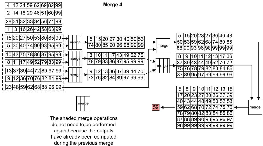
Figure 8-12 Merging 7 vectors for fourth median pixel
