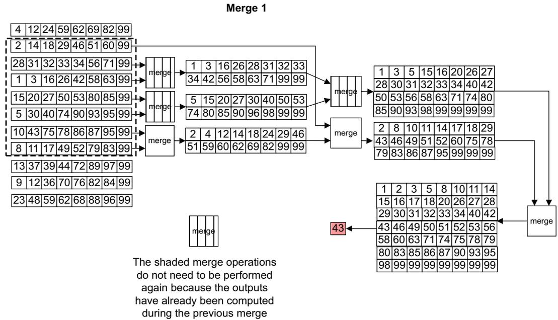
Figure 8-9 Merging 7 vectors for first median pixel
