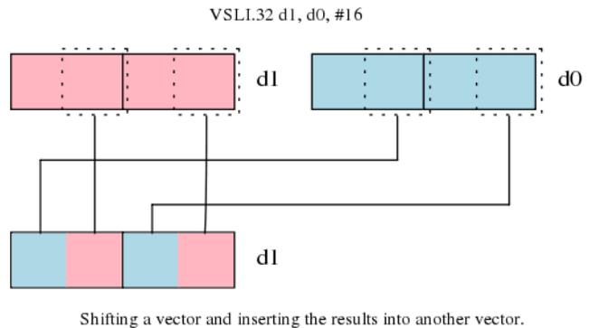
**Figure 3-6 Shifting and inserting**
